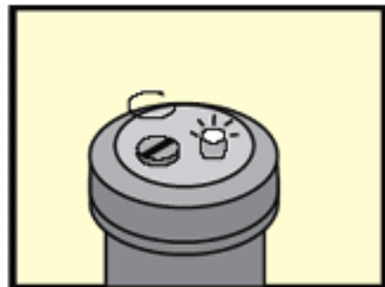
3.Check that LED light is on and replace cover
